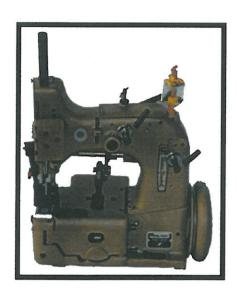
Pictured is the model 80700C bag closer. It is often used for sewing velcro to the back of artificial turf. The 80700C has both top and bottom feed for feeding the material uniformly through the machine. The 80700C is often used on a cart such as the one pictured above. The 80700C is also often used for various geotextile applications.
