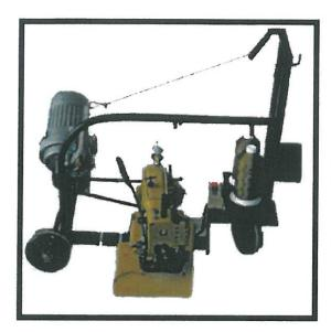
The model 81500T turf sewer makes a butt-seam for joining artificial turf as well as turf padding. The machine has both top and bottom feed dogs to keep the material feeding evenly through the machine. The model 81500T produces a butt-seam that can be pulled out flat and brushed down in the face of the turf.
