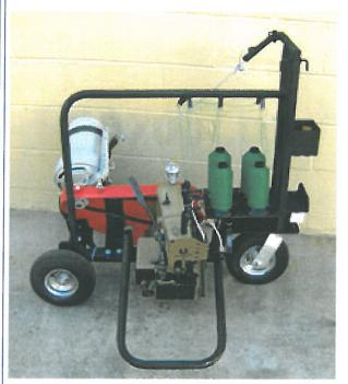
The model 80700CD3 is a two-needle four-thread bag closer. The 80700CD3 produces two parallel seams at a disctance of 7.2 mm just over 1/4". The 80700CD3 has both upper and lower feed dogs for postive feeding of the material. It is normally used for sewing the selvedge edge of sand or rubber filled turf. The machine sews a double locked stitch. It is pictured here on a TC815 turf cart with blower assembly. The blower assists in keeping the turf pile out of the seam during sewing.
