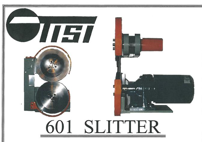
The model 601 slitter is designed for slitting heavy weight carpets and textiles at high line speeds. The 601 slitter is based upon a twin blade scissors action principle of cutting. One blade is positive driven and one blade is frictional driven, so any width material may be slit.
